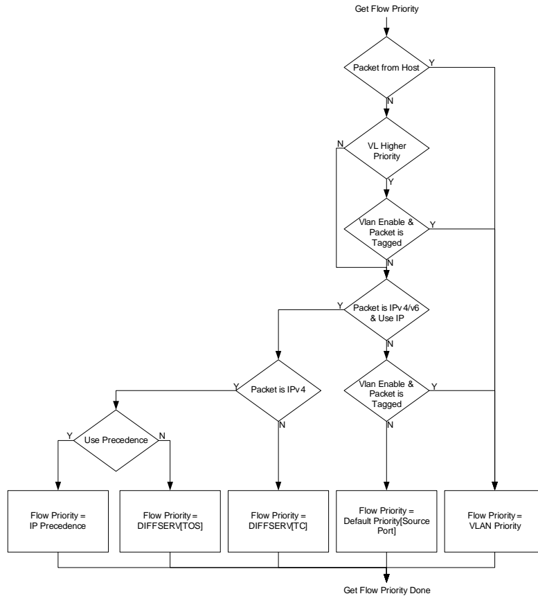
Figure 6.8 Switch Engine Ingress Flow Priority Calculation
